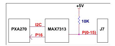
Port 16 of the MAX7313 is configured as an interrupt, so that any I/O Expander GPIO pin configured as an input can cause the PXA270 to be interrupted on GPIO1. These can also be used as PXA270 wake-up sources from sleep mode.
